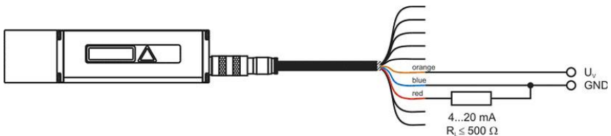
Figure 20 : Wiring diagram of analog output
