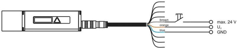
Figure 22 : Wiring diagram of trigger input
