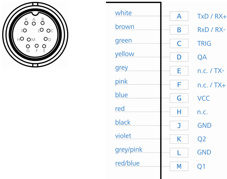
Figure 9 Connection drawing of the main connector
